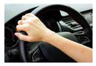
What's wrong with that? Well, if the airbag deploys in that position it may break the driver's arm or dislocate their elbow. Another problem is that it limits the driver's
